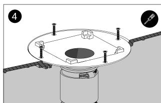
Firmly push the drain into position and screw the stainless steel screws into the shower base. Remove any excess caulk.
