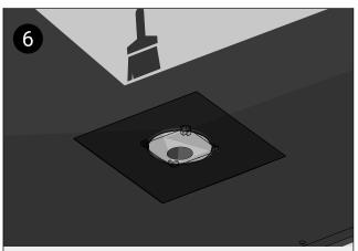
Completely cover the gasket with another layer of waterproofing membrane and then proceed with covering all the shower base area and any edges.
