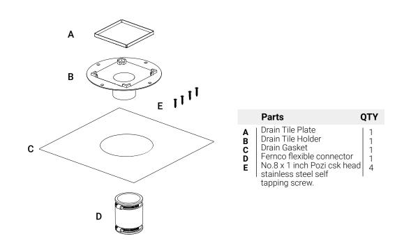
Suitable for wooden and solid floor installations. Use these in accordance with the former instructions. Do not use silicone caulk as this does not bond with the waterproofing compound. Only use acrylic caulk in waterproofing areas.
