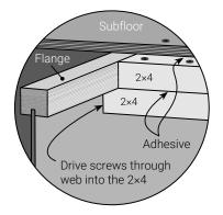
Install the perimeter blocking so that half of the block is under the subfloor and half is exposed.
