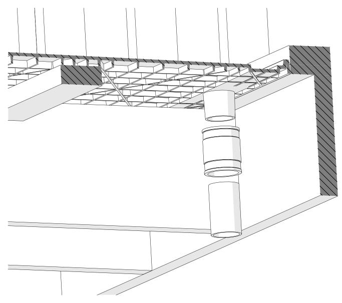
Note, the drain support blocking is not shown here for clarity.
