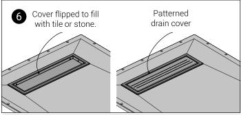
If you prefer to fill the cover, first rough-up its inside surfaces with 80 grit sandpaper, then clean them with a damp cloth. After it's completely dry, brush a coat of Tank/10® waterproofing onto the steel (to improve mortar adhesion). Use a modified thinset mortar to bed your tile or stone into position.
