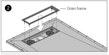
Insert the drain frame bolts into the threaded holes located at each corner of the gully.
