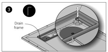
Adjust the bolts until the drain frame is level with the height of the tiles (use a hex driver if necessary). When it comes time to tiling, you'll want to pack thinset mortar under and around the drain frame once you have its elevation set.
