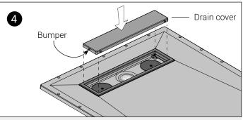
Insert the six bumpers into holes in the edges of the cover (if needed, taper the bumper stems with a utility knife and add a drop of dish soap to insert them), Lower the drain cover into the drain frame.
