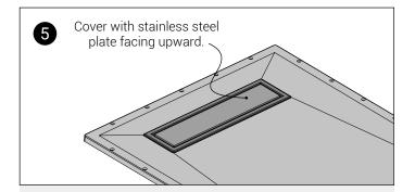
You can install the drain cover so it's on display, flip it over and fill it with tile or stone or even use the decorative patterned drain cover.
