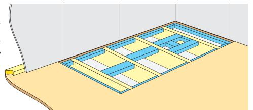
Once you have the blocking thoroughly installed, cut a 1/2"-thick panel and dry fit it on the framing. Check it for level and for the consistency of support - you want a tight fit between the framing and the panel. Most importantly, the base must be level and this is the time, with the framing exposed, to make adjustments to ensure that result. When you're confident that the framework is properly prepared, apply construction adhesive to all blocking and joists.
