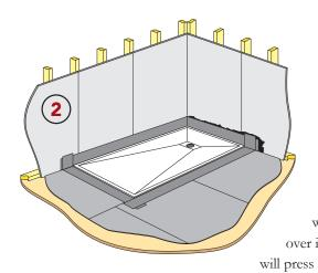
making sure it remains wet before you press the tape into it (some types of tile backer board absorb liquid waterproofing very fast, so you may have to recoat the surface several times before it remains wet — glistening — when you reposition the tape). Return tape to the wall and brush Tank/10 over it throughly. Brushing will press the tape into the com-
