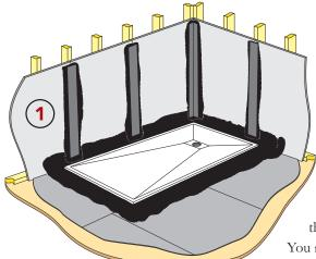
After embedding all the flange tape around the shower base turn your attention to waterproofing the joints between wall board panels. The trick with waterproofing is to work from the back of the shower to the front as much as possible. This progression helps keep you from stepping into wet and sticky material.
