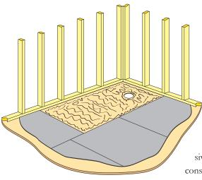
Install tile backer board or uncoupling membrane on the subfloor outside the shower base installation area. Follow manufacturer's instructions for the installation of their product. Leave a narow gap of about <sup>1</sup>/<sup>1</sup>/<sup>16</sup>" around the shower base area to accommodate the flange tape that will be installed later. If you need to position the shower base on the subfloor to act as a guide while installing the tile backer board or uncoupling membrane, please do so.
