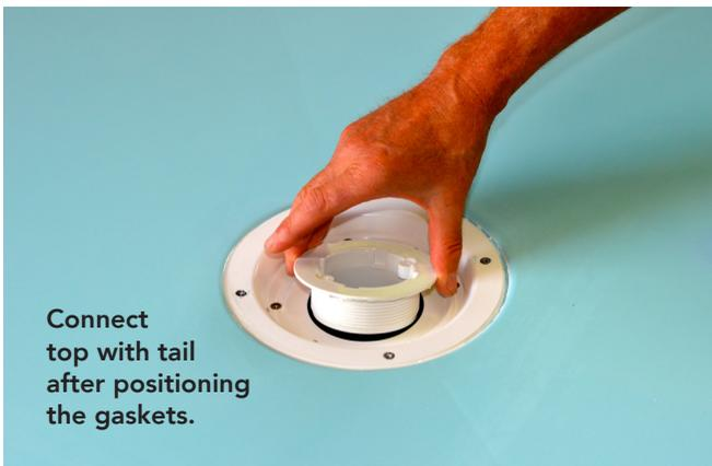
Connect top with tail after positioning the gaskets.
